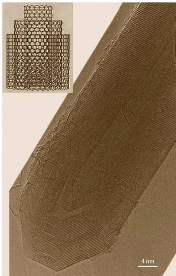
Fig. 3.5 High-resolution transmission electron microscopy image (longitudinal view) of a concentric multiwall carbon nanotube (c-MWNT) prepared using an electric arc. The insert shows a sketch of the Russian-doll-like arrangement of graphenes
