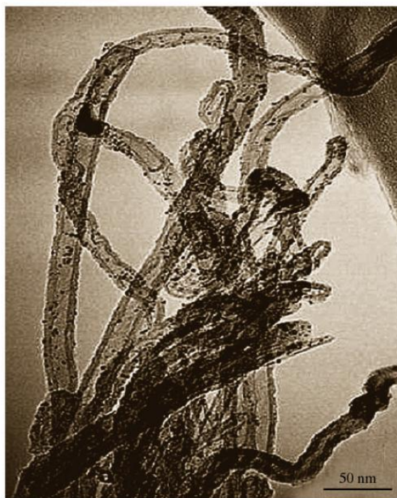
Fig. 3.31 Transmission electron microscopy image showing rhodium nanoparticles supported on the surface of an MWNT (from [3.329]) ▶
