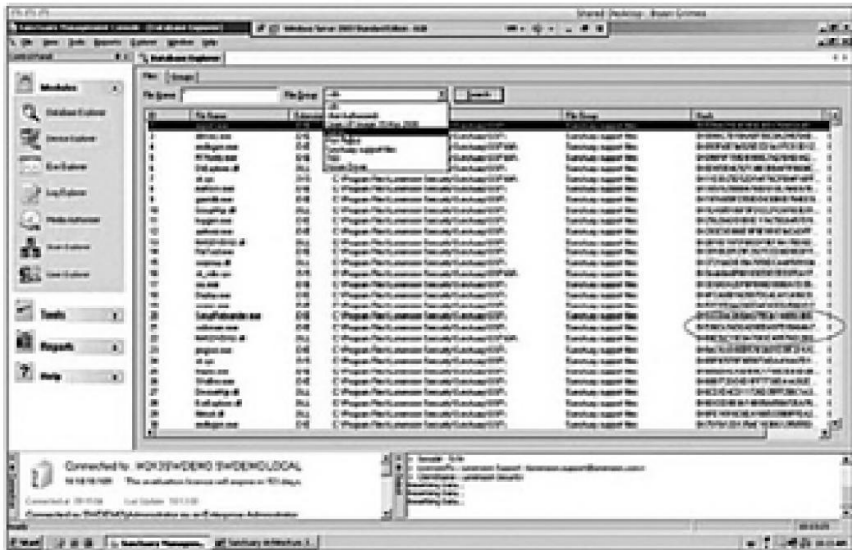
Figure 1.5 A unique SHA-1 signature is calculated for each binary file, together with the filename, path, size, and product version. This information is recorded on the Lumension server whitelist, defining what programs can run on all selected computers.
