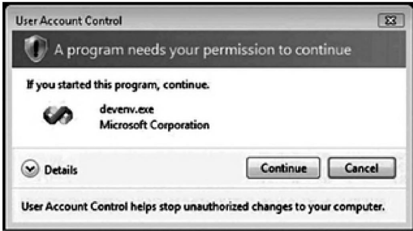
Figure 1.12 An example of the annoying interruptions provided by UAC is the pop-up received when a user would attempt to run any program with administrative privilege.
