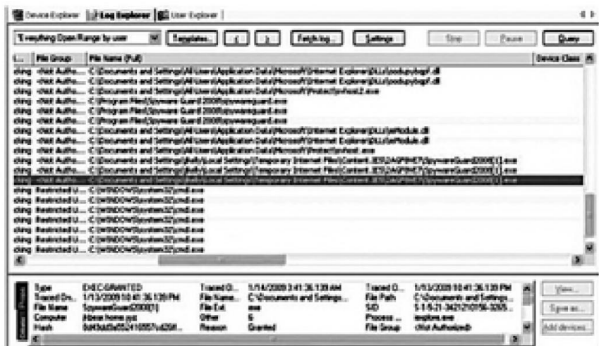
Figure 1.10 Positive security model-based application control automatically blocked the operation of the rogue software executables because they were not part of the permitted applications that the user had administrative permission to execute.
